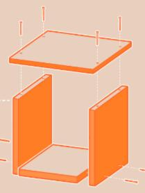
Attach the back shelves to the side panels using eight short nails as shown.
