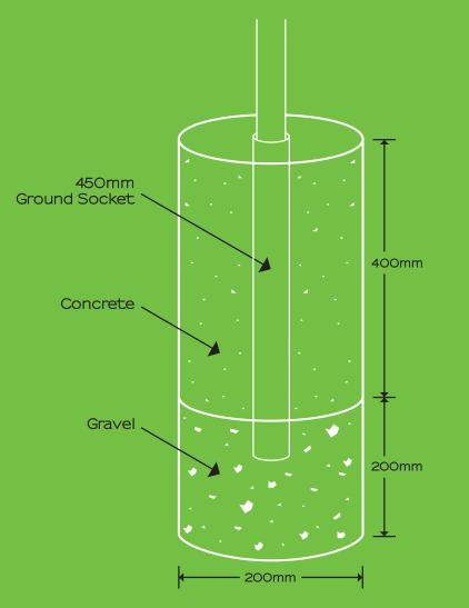
3. Ensure when installing the ground socket that it is firmly located in a vertical position.
