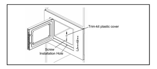
Open the door. Fix the oven to the cabinet with a screw through the installation hole at the front of the trim kit. Once in place, fit the trim kit plastic cover into the installation hole.
