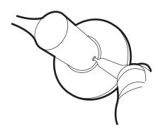
Depress button and slide off handle of chassis
