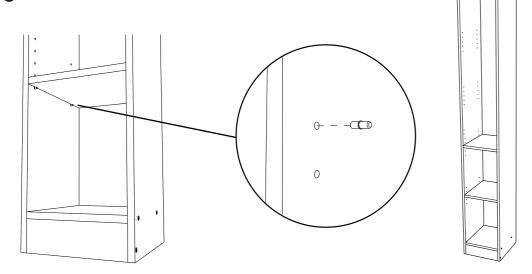
7. Fixing the Rail Brackets to the Tower and End Panels.
