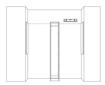
\* **Note:** Fixing Tower and End Panels to unsupported Gib is not recommended.
