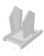
3. Install body panel on the base with x4 short nails.
