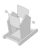
4. Slide x2 windows into slots. Install the screw eyes on body panel of both sides.
