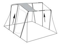
12. Assemble the porch ridge pole (Part #10/2 and #50) and connect to the opening in Part #2/1 at the centre of the front of the tent. Carefully, pull the porch canvas out over the assembly and vertically place the Porch Centre Pole through the eyelet of Part #10/2 and then the porch canvas. Then guy rope this directly out.
