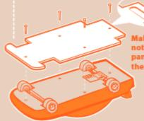
Make sure the notch in the panel is facing the motor.
