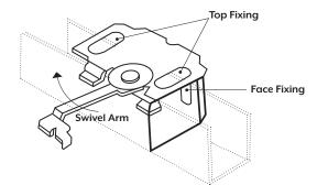
3. Now present the Blind to the Bracket ensuring that the Lugs are positioned snugly under the front rim of teh Headrail. Then push the Locking Arm until it's pressed against the Headrail.
