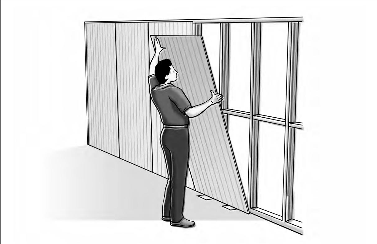
**Figure 5: Sheet fixing**
