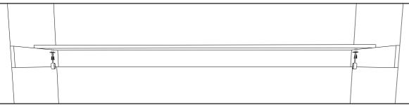
Make sure to fix End Supports as far forward as possible, so that your coat hangers fit accordingly.
