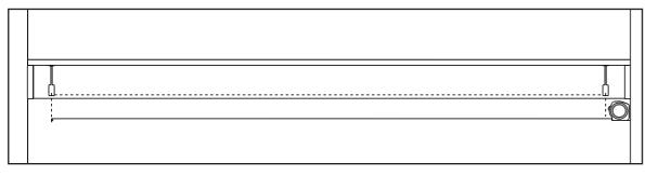
2. Using your tape measure, measure this distance on your rail and trim using a hack saw.
