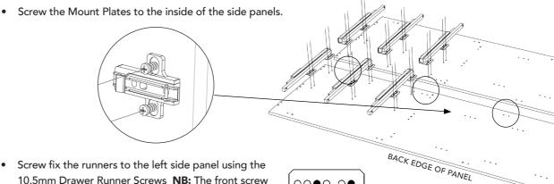
10.5mm Drawer Runner Screws NB: The front screw position is 3 holes back from the front of the runner.
