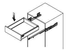
Slide out the slides, and place the drawer in from above onto slides.
