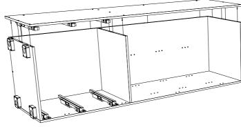
• Flip the cabinet over to fix the last side panel to the base, back and top panels using 50mm Cabinet Screws.
