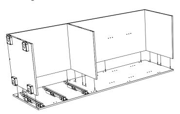
base, fixed shelf, back, and top panels ensuring the holes align with the dowels. Fasten with the 50mm Cabinet Screws.
