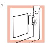
Next put the external frame (main body into the hole from the exterior. Place the internal frame from inside onto the external frame.
