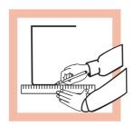
Position the template at the appropriate height with the bottom of the pet door level (where practical) with the pet's stomach. Tape the template to the door or panel that you are installing into. Ensure the template is level. With a pencil trace the line to be cut.
