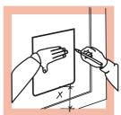
Drill four 10mm holes in the corners as per the diagram shown, making sure that the corners are the centre point of the hole.
