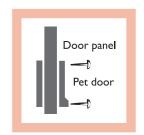
Ensure the screws provided are cut to the correct length. The correct length is door panel thickness plus 12mm.
