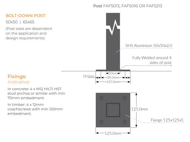
**4.2** Fix the posts in place with four fixings of the correct type for the situation.
