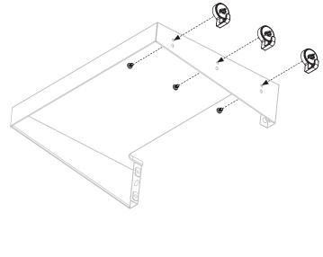
**STEP 09** Slide the right side shelf step bolts onto the side shelf brackets. The threaded M8 step bolts will hook and hold the shelf. Use two (2) M8 step bolts [e.] to secure the shelf to the griddle body by screwing them into the bottom hole of the brackets. Repeat this step with the left side shelf.
