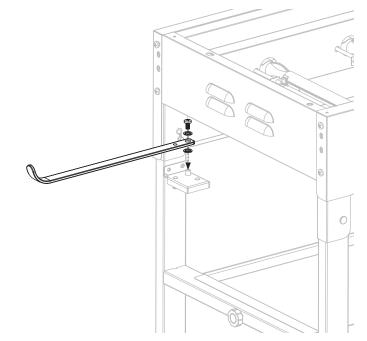
**<u>STEP 06</u>** Use four (4) M6x12 bolts [**a**.] to install the side handle to the left side of the griddle body.
