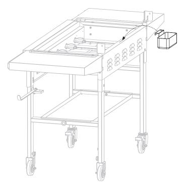
**STEP 11** With the help of another person, place the griddle top and hood on the main body by aligning the 4 pins to the holes of the body.
