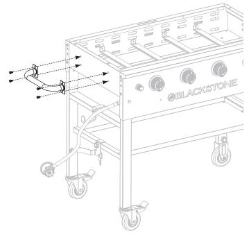
**STEP 07** Use four (4) M6x12 bolts [a.] to attach one (1) right front side shelf bracket (L), and one (1) right rear side shelf bracket to the right side of the griddle body.
