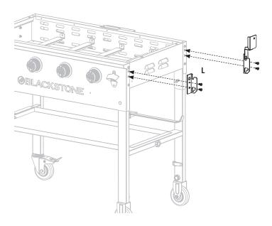
**STEP 08** Use the three (3) M6x8 screws pre-installed in the shelf hooks to attach three (3) shelf hooks to the left side shelf.
