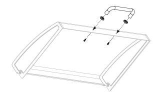
**STEP 13** Place the hood on the griddle top and align the holes with the rear side shelf brackets. Use two (2) M8x19 bolts [f.], two (2) washers [g.] and two (2) M8 nuts [d.] to attach the hood to the rear side shelf brackets.
