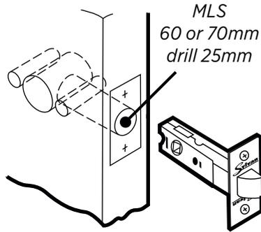
**3 Fit spindle through latch**
