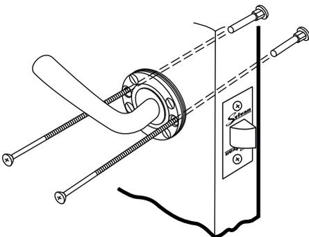
**5 Drill and fit 4 wood screws for alignment only**
