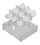
4. Place the blocks inner assembly into frame.
