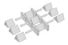
3. Assemble the blocks with inner panel (A) and wooden rods.
