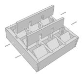
6. Insert x2 inner panel (B) parts into slots. Secure with x2 nails on each side.
