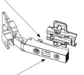
• Push the back down onto the hinge mount until you hear a click.
